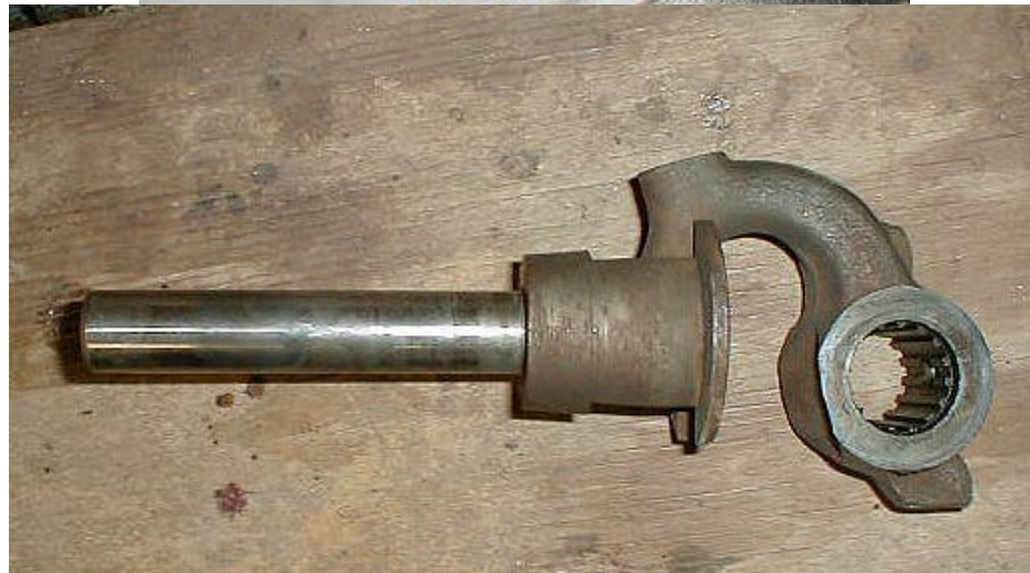
Inner shock absorber cam.
