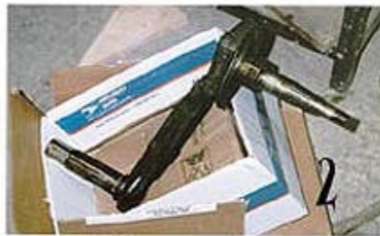
One end of the main shaft is worn by the needle bearings.
