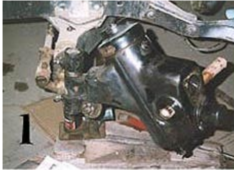
Picture #1 is the knee action unit on the car. The main shaft below is removed.
