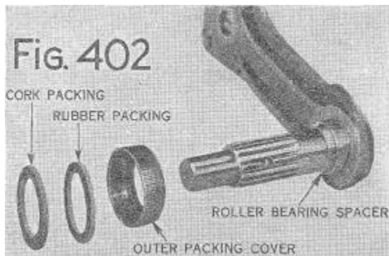
Fig. 402-Component parts of the support arm assembly.
