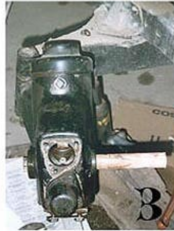
Above is a top view, with a piece of wood I used to "follow" the main shaft.
