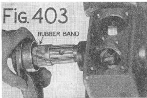
Fig. 403- Use a rubber band to hold needle rollers in place when installing the support arm.
